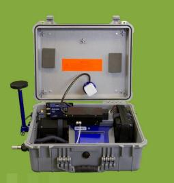
The DustTrak™ II and DRX Aerosol Monitor Models 8530, 8530EP, 8533 and 8533EP are portable, battery-operated, laser-photometers that measure and record airborne dust concentrations.
