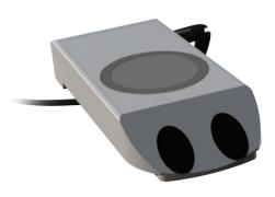
This sensor is used in open channels or pipes that run partially full. This sensor is used to measure depth (using a capacitive pressure diaphragm) and velocity. Access to the monitoring point is required for installation and maintenance.
