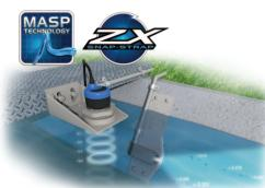
This sensor is used to measure velocity only in full pipes when access to the pipe is available and the pipe can be emptied when installation or maintenance is required. It can also be used in partially full pipes or open channels in situations where the user is measuring depth by a third party or ultrasonic depth sensor.
